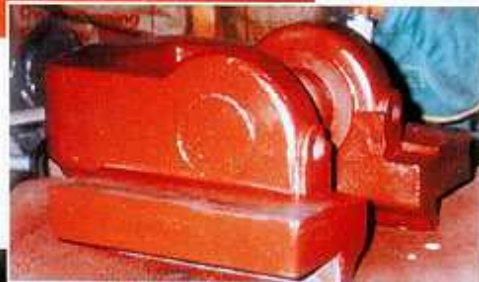
Crosshead after pouring new babbitt (above) and after a coat of primer (right). A freshly babbitted and primered bearing cap (below).
