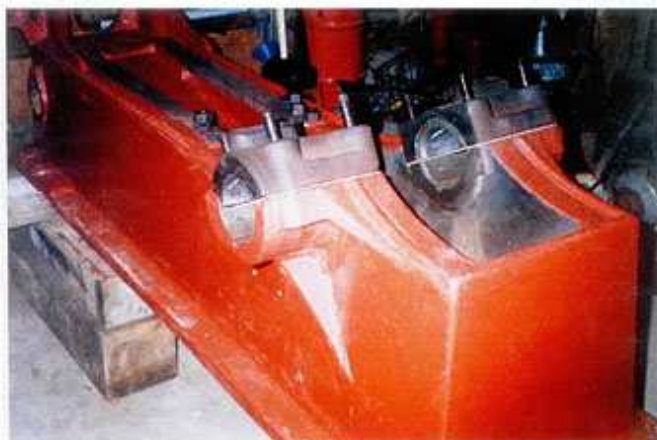
The Swan's bedplate and main bearing caps are fitted and ready for rebabbitting.
