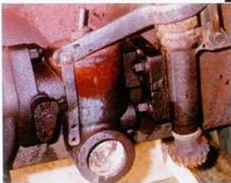
Above: Mixer and governor before disassembly.
